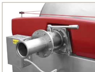
overfilling signalisation, axial filling valve
