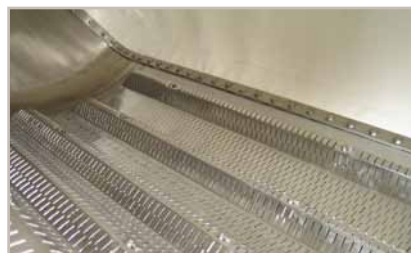
connected draining channels, electropolished
